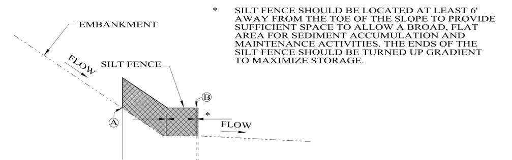
**SILT FENCE SECTION AT TOE OF SLOPE**
