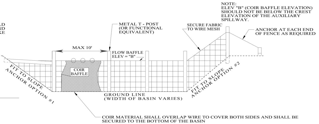
FLOW BAFFLE DETAIL
