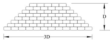
**SAND BAG PLUG & BERM CROSS SECTION
