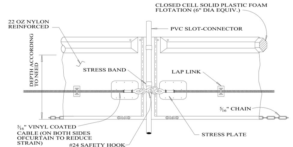
TYPE 3 CONFIGURATION SHOULD BE USED IN AREAS WHERE CONSIDERABLE CURRENT ( $\leq 5'$  PER SECOND) MAY BE PRESENT, WHERE TIDAL ACTION MAY BE PRESENT, AND/OR WHERE THE CURTAIN IS POTENTIALLY SUBJECT TO WIND AND WAVE ACTION.
