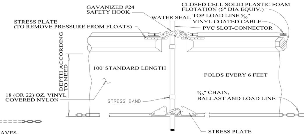
TYPE 2 CONFIGURATION SHOULD BE USED IN PROTECTED AREAS WHERE THERE MAY BE SMALL TO MODERATE CURRENT RUNNING ( $\leq 3.5'$  PER SECOND) AND/OR WIND AND WAVE ACTION CAN AFFECT THE CURTAIN.
