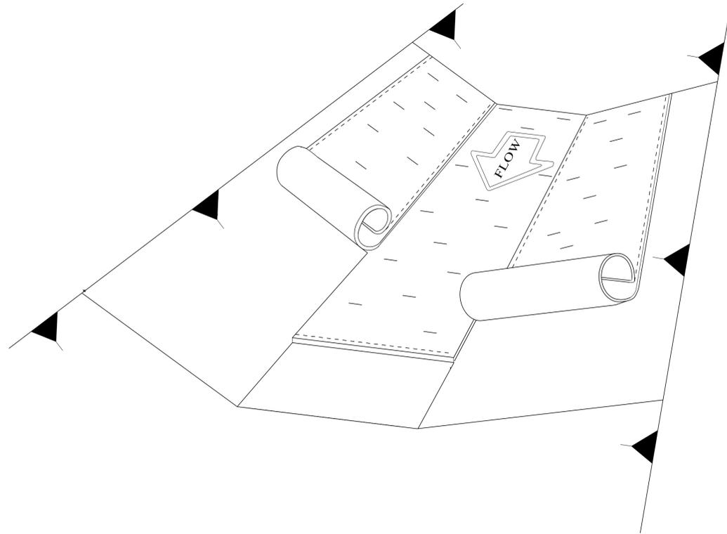
**SLOPE INSTALLATION DETAIL**
