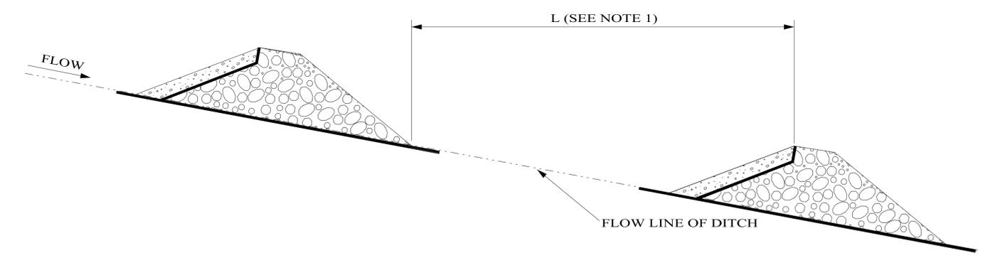
DETAIL FOR SPACING BETWEEN DITCH CHECKS
