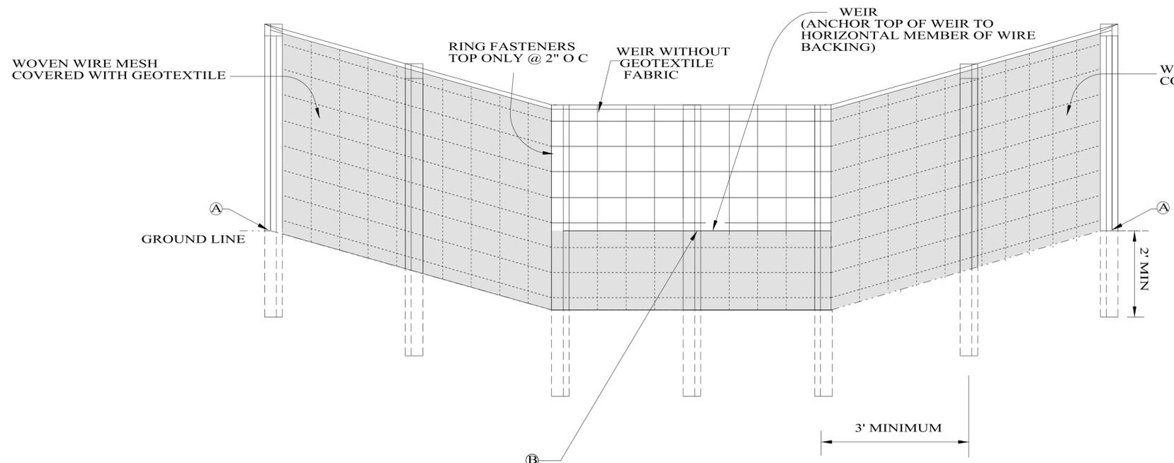
NOTE: END POINTS **A** MUST BE HIGHER THAN TOP OF GEOTEXTILE AT POINT **B**
